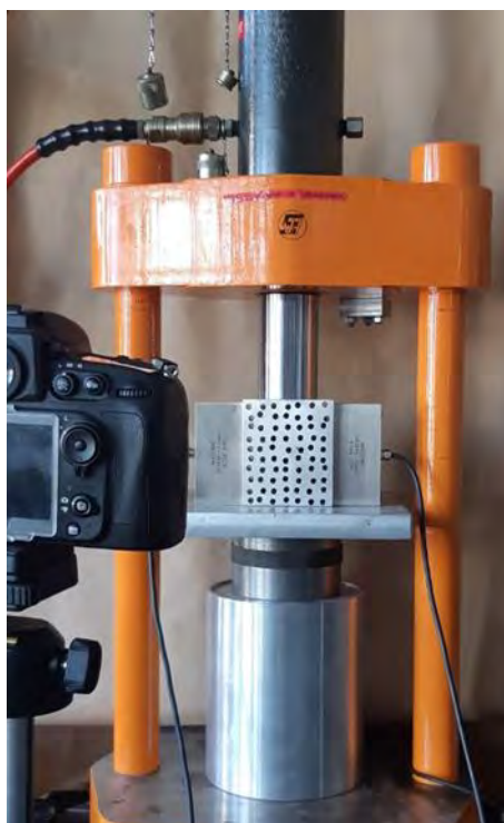
Figure 9 Image of the experimental apparatus. The piston of a servo controlled 10 T press loads a holed block of Au4G (70 holes of radius 3 mm). Two linear acoustic arrays of 32 sensors are held in direct contact with the boundaries of the sample.
