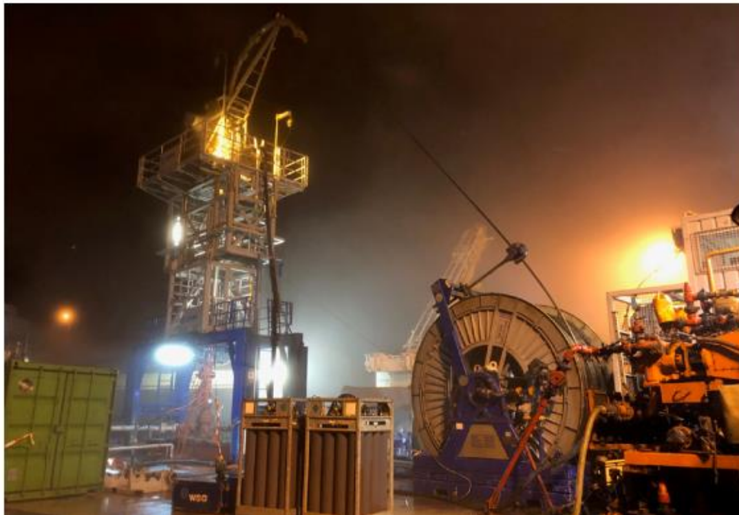
Image: Soultz-sous-Forêts geothermal site by night during the chemical stimulation done in the framework of DESTRESS project. Source: és Géothermie.
